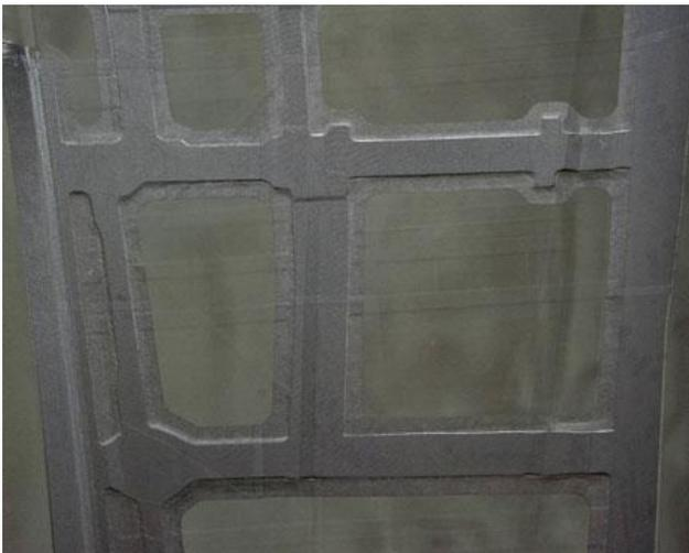
Figure 3 Routed Forward Fuselage Panel
