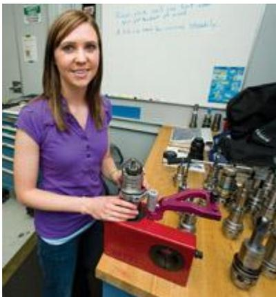
Machining countersinks used to be one of the more costly challenges of the process. Because of the precision that even countersinks require on the F-35 skin parts, technicians used to measure holes with manual countersink gages and update machine offsets manually. The procedure was time-consuming and error-prone. Now, the manual work has been eliminated using a device Lockheed Martin developed internally. The device is the PINC, for pressure induced normal-vectorized countersink.
