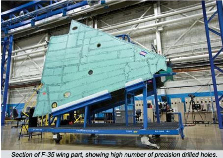
Section of F-35 wing part, showing high number of precision drilled holes.
