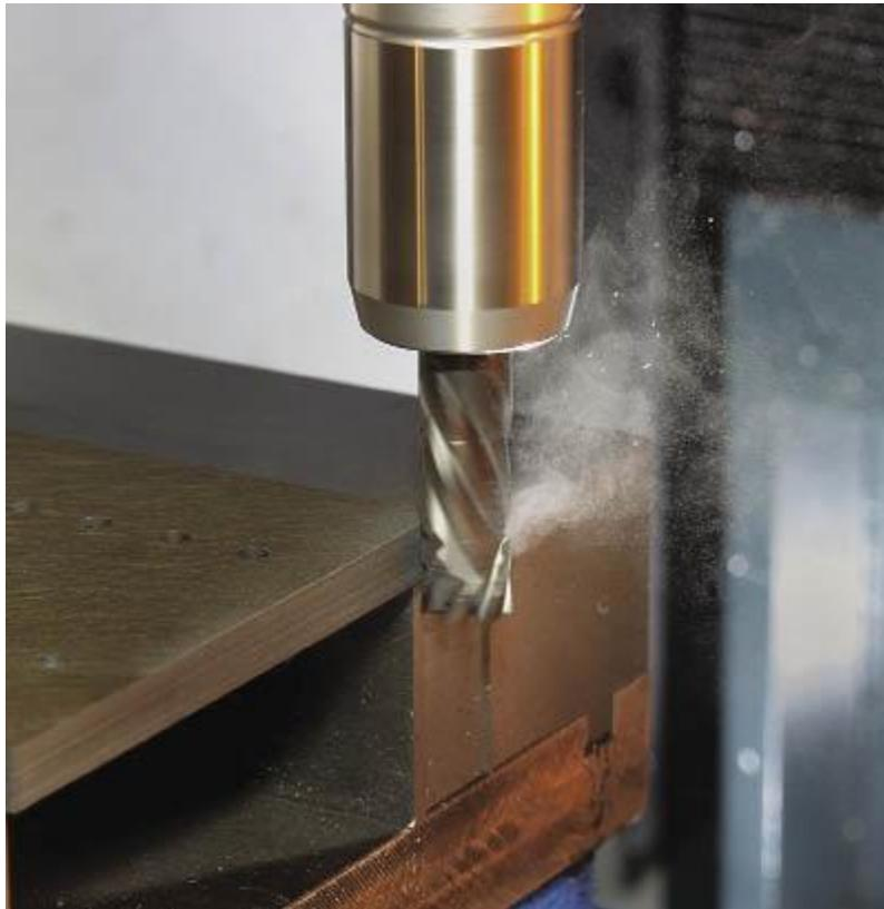
*Compression router trimming edge of composite panel*
