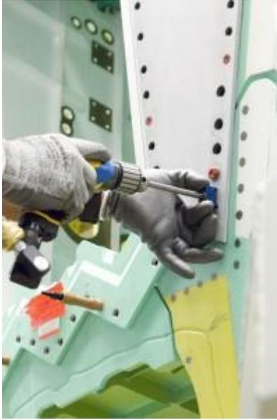
Users of custom tools may also benefit from step production. Rather than use multiple tools for different steps in machining, the machinist can employ one custom tool for multiple operations — drilling, reaming and cold-forming a part, for example.
